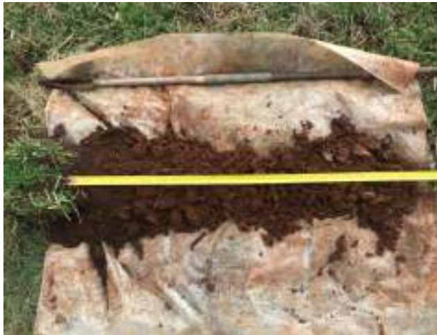
Soil profile captured on 2 July 2020 from TP2, topsoil is at the left of the photo
