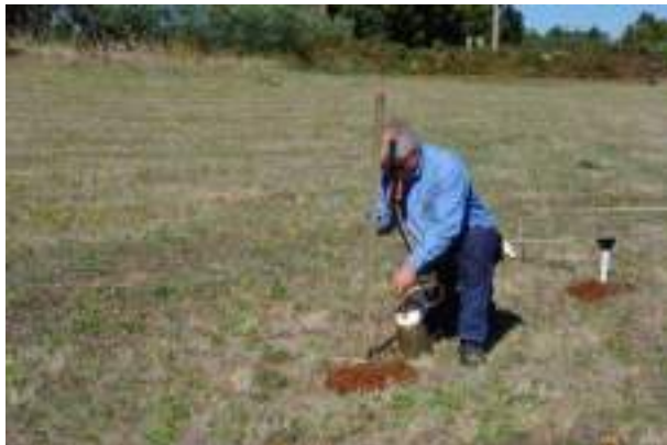
Extracting excess water from the hole
