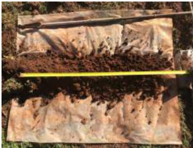
Soil profile captured on 7 July 2020 from TP1, topsoil is at the left of the photo
