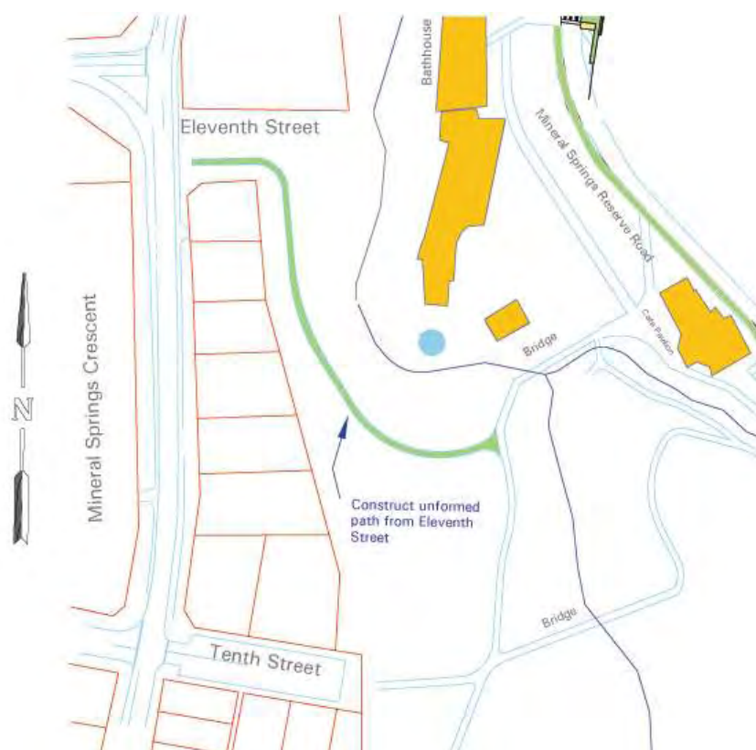
Figure 3.9 Construction of path from Eleventh Street
