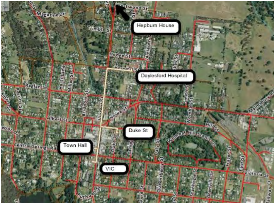
Figure 3 - Boiler located at Town Hall. Total Pipe length 1120m. Hepburn House could be an additional site
