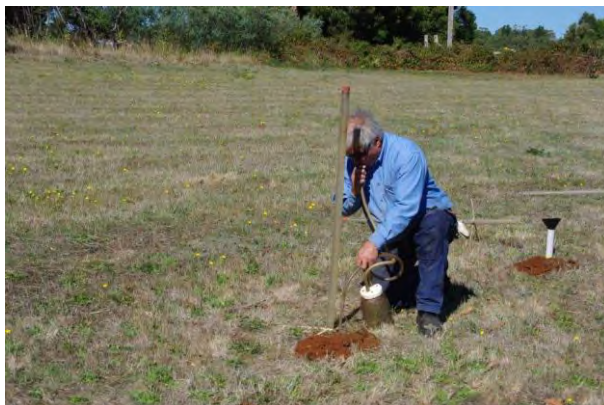
Extracting excess water from the hole
