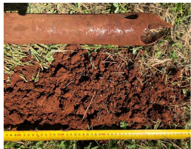
Close-up of the bottom of TP1, sub soil BC
