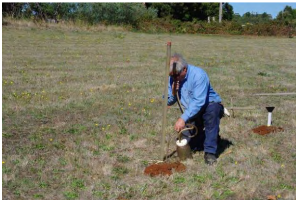
Extracting excess water from the hole
