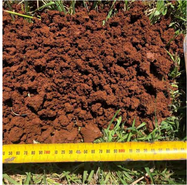
Close-up of the bottom of TP1, sub soil BC
