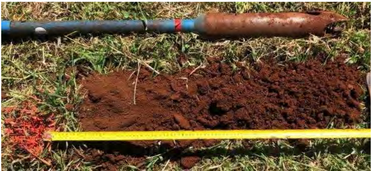
Soil profile captured on 31 October 2021 from TP1, topsoil is at the left of the photo
