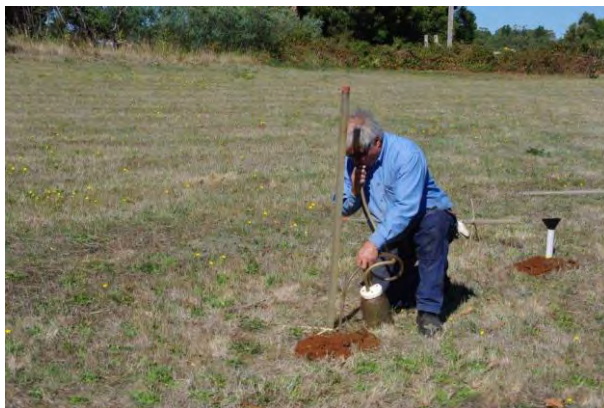
Extracting excess water from the hole
