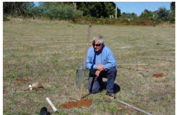
The drop in water level was recorded at three minute time intervals
