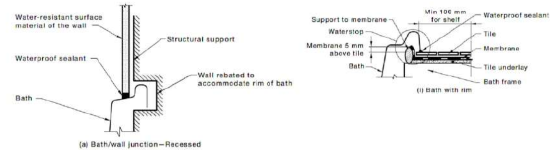
TYPICAL BATH JUNCTION DETAIL
