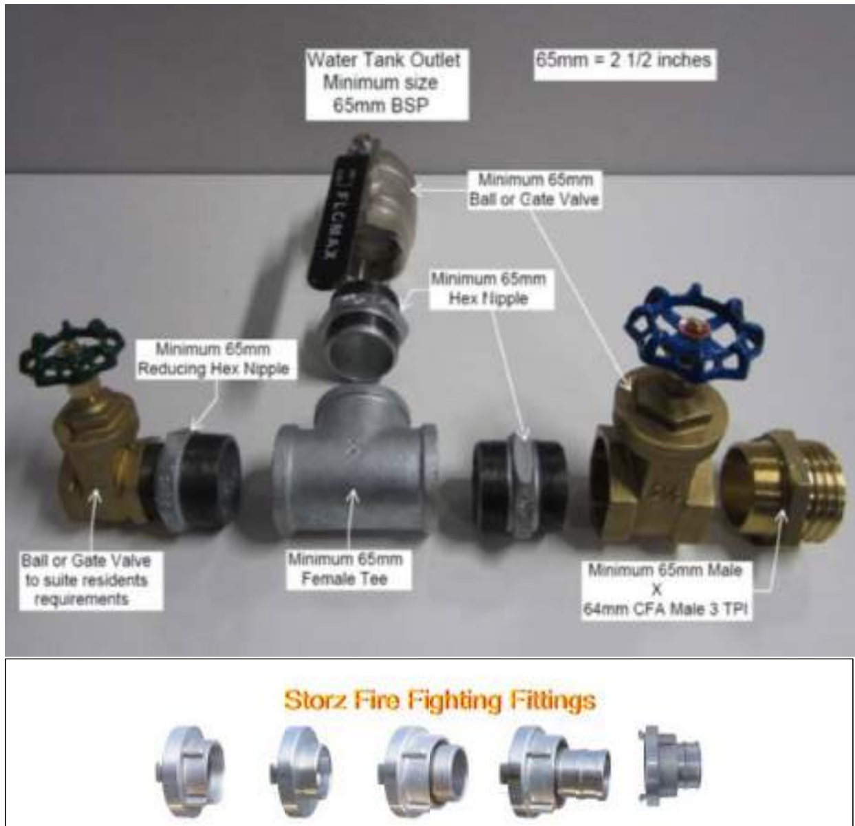
Diagram 1 CFA Standard permit conditions for water supply, in FRV areas pls check if they use same fittings or Storz Fitting apply.
