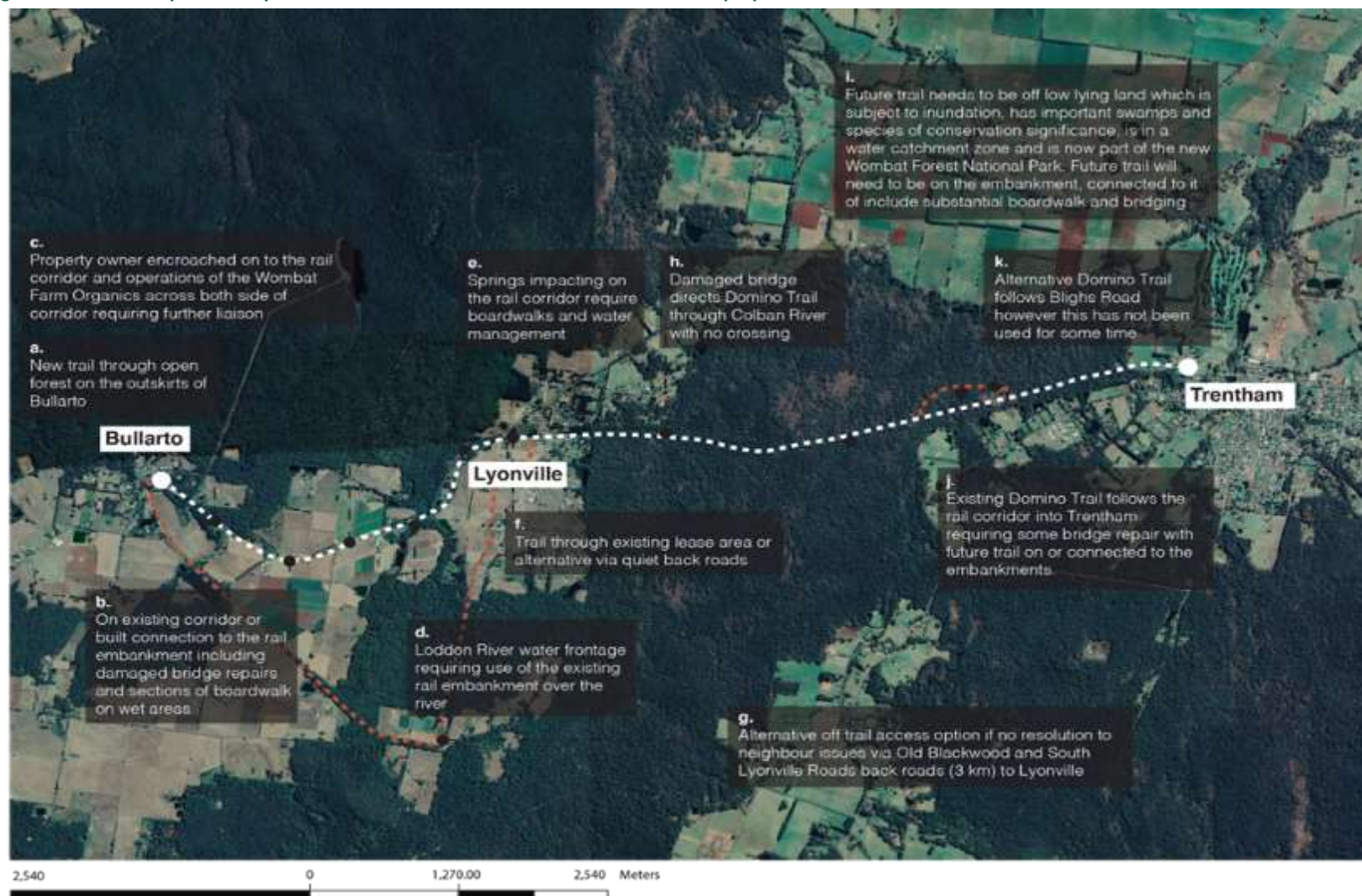
Figure 5. Issues and options analysis between Bullarto and Trentham where DSCR have proposed a tourist train extension
