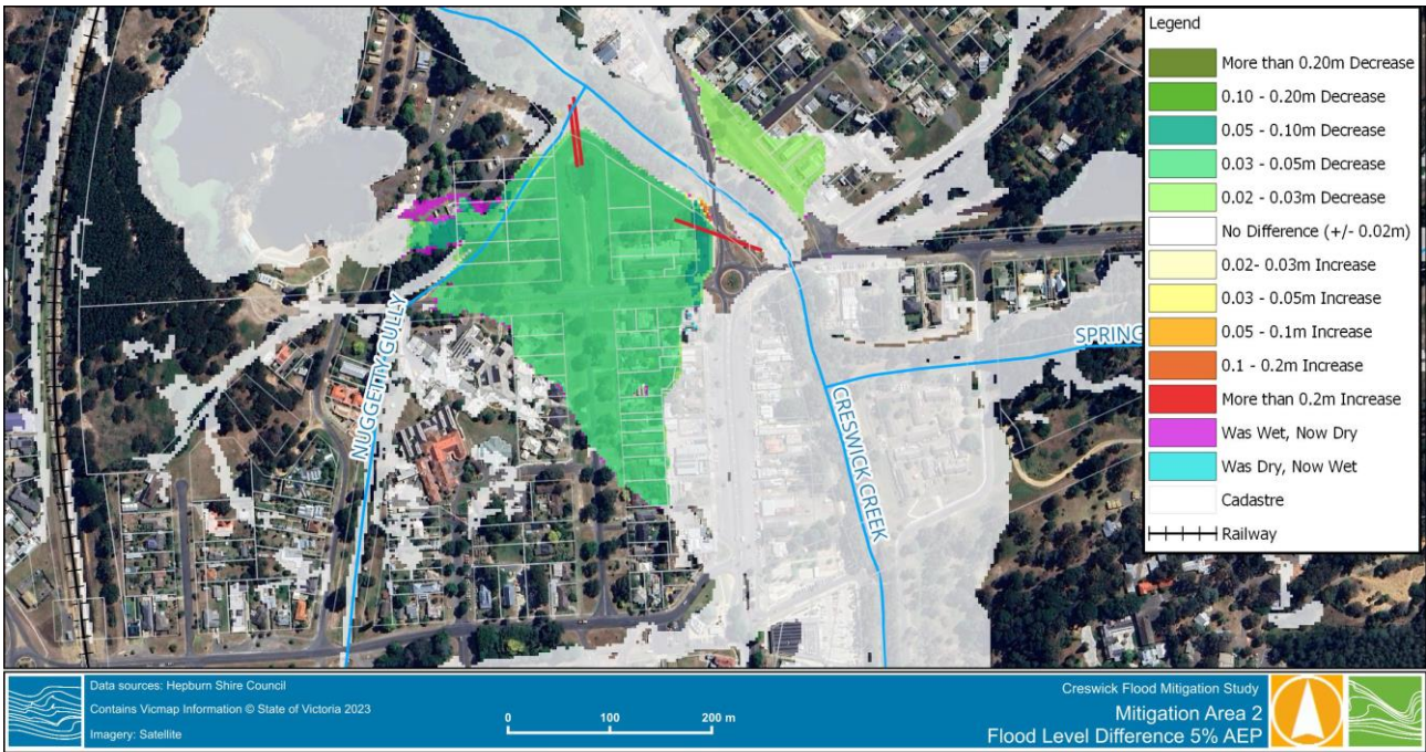
Figure 8-10 Mitigation 2 – 5% AEP Flood Level Difference
