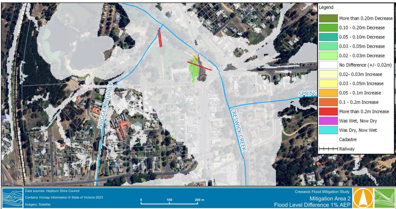
Figure 8-11 Mitigation 2 – 1% AEP Flood Level Difference
