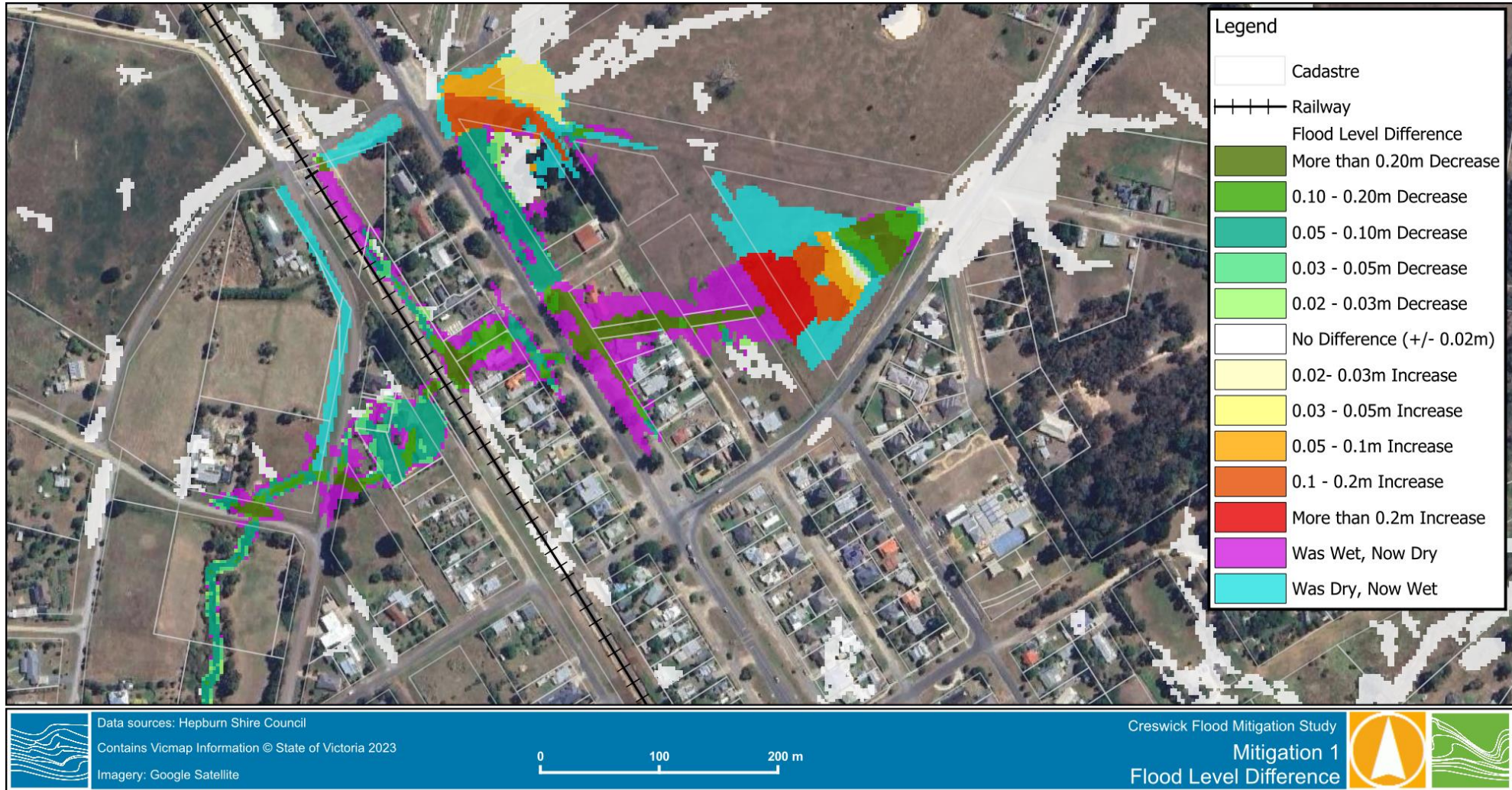
Figure 8-3 10% AEP Flood Level Difference Plot – Location 1
