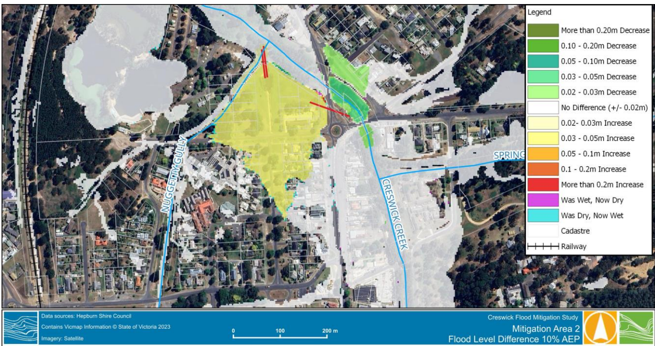
Figure 8-9 Mitigation 2 – 10% AEP Flood Level Difference
