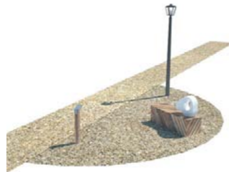
Typical sculpture node incorporating; Street lamp - possibly off-grid Compacted gravel surface with integrated pad footing Steel edge to gravel
